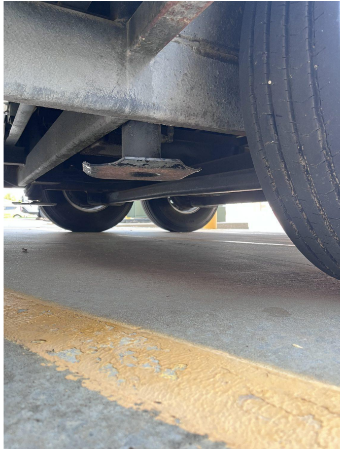
Underbody/frame view shows back feet for Big Foot Level system
