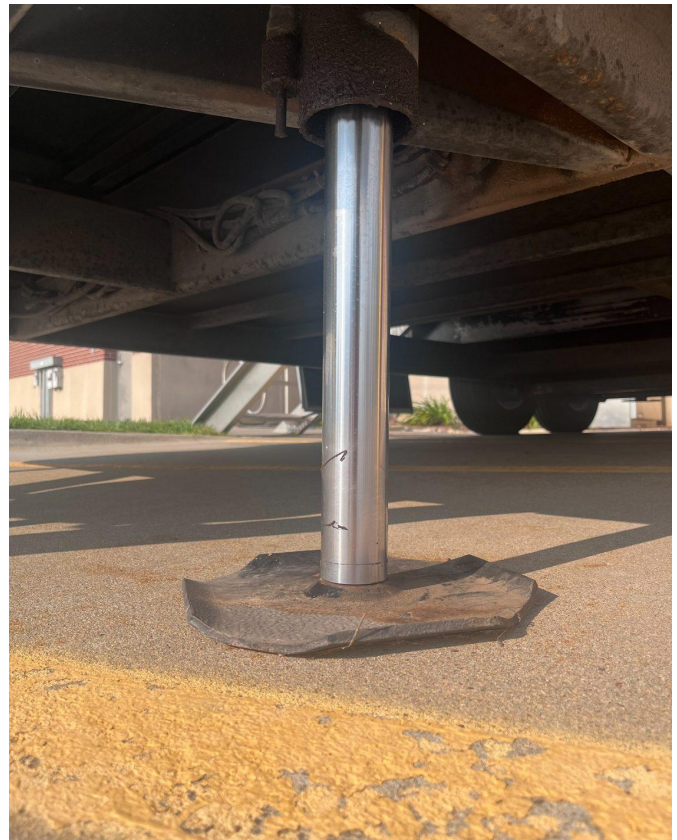
One of the four hydraulic parking/stabilizing feet shown extended.
