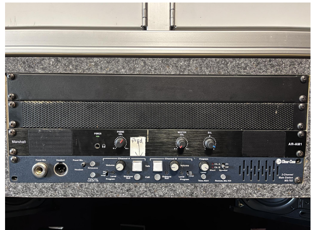
Clear-Com MS-702 2-Channel Main Station with Marshall AR-AM1 above the audio-board position.
